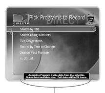
If the DVR is low on Program Guide Data, this message at the bottom of the screen tells you how much Program Guide Data it has.
